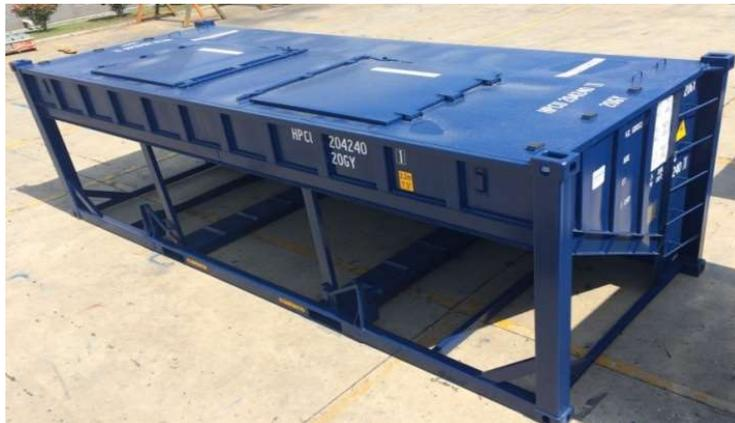
**Equipment Container for installing power generator**
